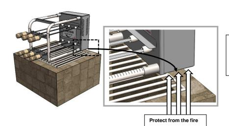
**9.** When installing the CARSON KIT - CRK6 make sure that the Main Case gets as minimal exposer to direct flame as possible. See the fire pit assembly example to the left..
