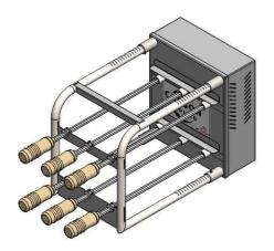
**8.** The Pulley slides on the skewer blade. After defining the position set screw with the allen wrench 1/8 "
